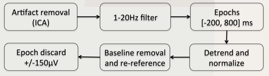
Figure 5. EEG offline processing flow
